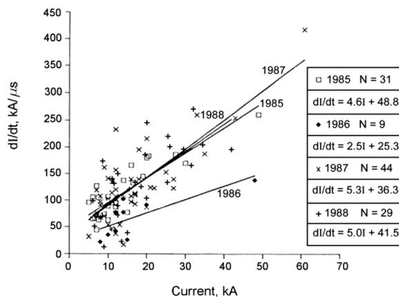
Fig. 6. Relation between the peak value of current rate of rise ( $di/dt$ ) and peak current from triggered-lightning experiments conducted at the NASA Kennedy Space Center, Florida, in 1985, 1987, and 1988 and in France in 1986. The regression line for each year is shown, and the sample size and the regression equation are given [39]
