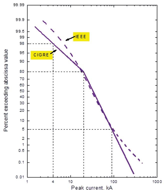
Fig. 2. Cumulative statistical distributions of peak currents for negative first strokes adopted by IEEE and CIGRE and used in various lightning protection standards [19]
