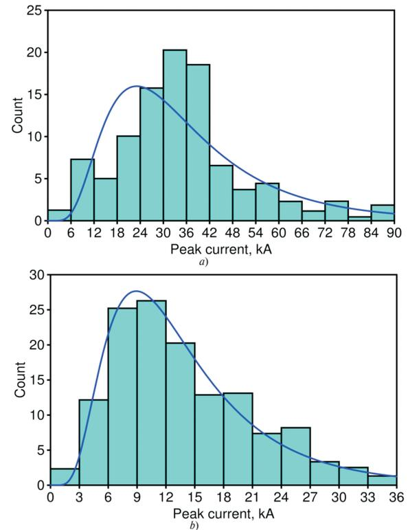
Fig. 9. Histograms of peak currents corresponding to cumulative distributions [4] for: a) negative first ( $n=101$ ) and b) negative subsequent ( $n=135$ ) strokes
