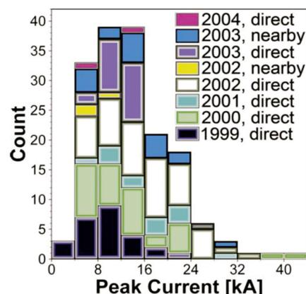
Fig. 4. Histogram of return-stroke peak currents for 165 strokes in rocket-and-wire triggered lightning flashes from Camp Blanding, Florida, 1999–2004 [32]
