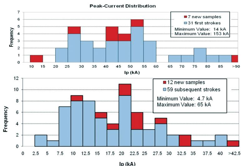
Fig. 3. Histograms of peak current for negative first (top panel; median value = 45 kA,  $n=38$ ) and subsequent (bottom panel; median value = 18 kA,  $n=71$ ) strokes from direct measurements in Brazil. Blue color corresponds to measurements in 1985–1998 and red color to measurements in 2009–2010 [70]
