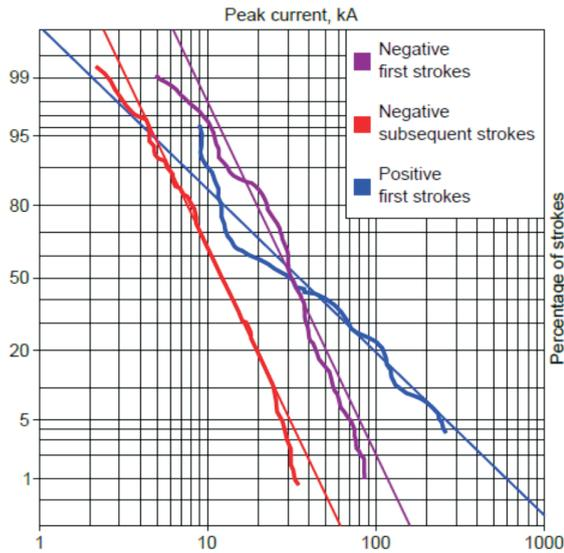
**Fig. 1.** Cumulative statistical distributions of return-stroke peak current from measurements at the tower top and their lognormal approximations (straight lines) for negative first strokes ( $n=101$ ), negative subsequent strokes ( $n=135$ ), and positive first strokes ( $n=26$ ) [4]
