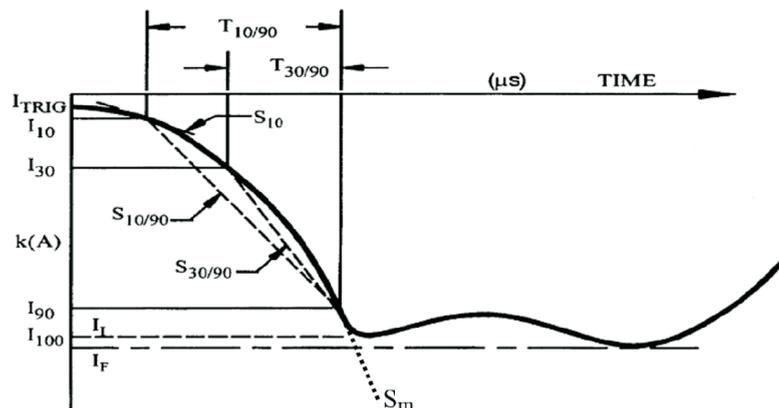
Fig. 5. Description of lightning current waveform parameters. The waveform corresponds to the typical negative first return stroke [3, 19]
