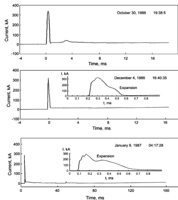
Fig. 7. Directly measured currents in three positive lightning discharges in Japan. Note the very large peaks, from top to bottom, 340, 320, and 280 kA, of the initial pulses followed by continuing currents. Transferred charges are 330, 180, and 400 C, respectively [48]
