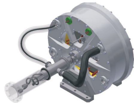
Fig. 14. HTS motor from GREEN and SAFRAN for aeronautic
