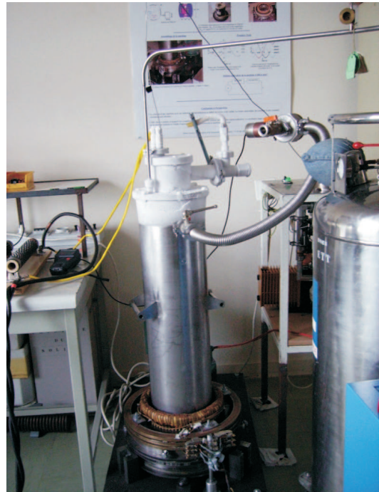
Fig. 13. Magnetic flux concentration with HTS bulks motor
