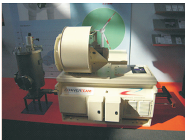
Fig. 9. 250 kW HTS motor realized by Converteam Nancy and GREEN
